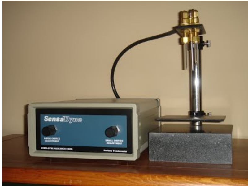
Figure 3.24. SensaDyne QC6000 Surface Tensiometer
