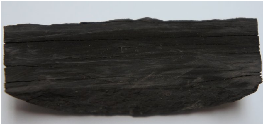
Figure 3.3. Bulk shale cracked when fluid is introduced
