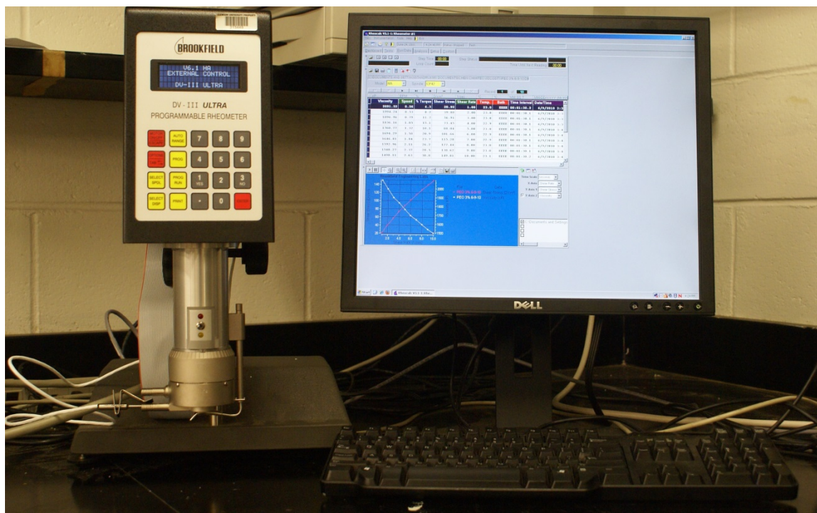
Figure 3.27. Brookfield DV-III Ultra Viscometer
