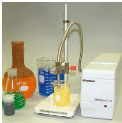
Figure 3.26. Nanotrac 250 particle size analyzer
