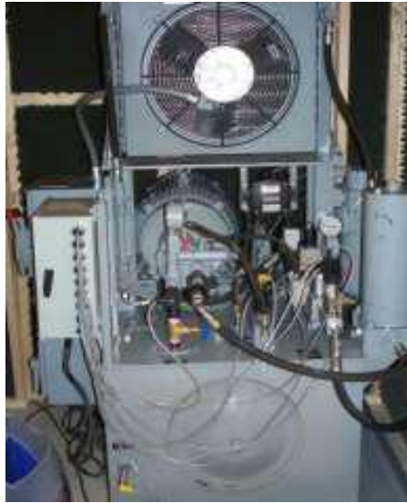
Figure 5.13. Picture of the axial piston pump testbed
