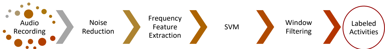
Figure 3.2: Machine learning model for audio signal processing.
