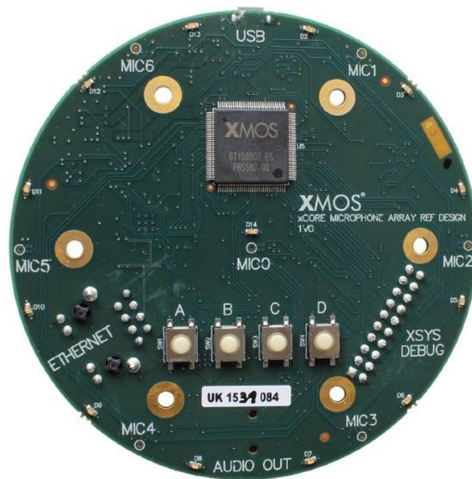
Figure 2.4: xCORE-200 microphone array evaluation board – top (XMOS Ltd. 2016).
