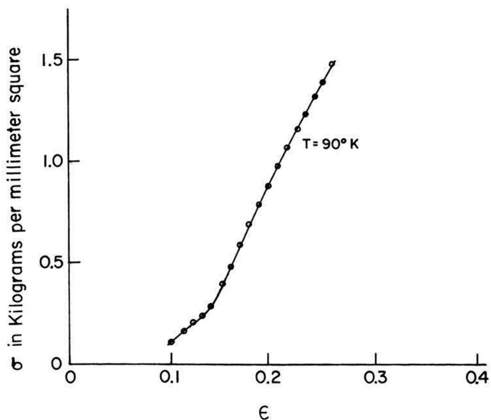
Figure 3 Work hardening of 99.99 percent Aluminum
