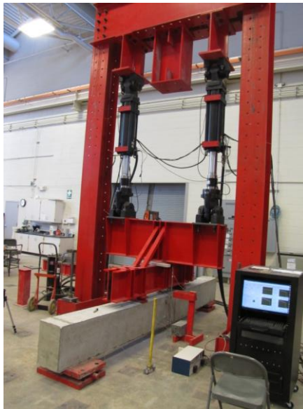
c) Splice test setup with specimen loaded
