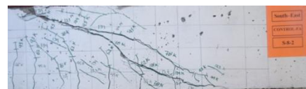
Figure 3 - Crack pattern of the beams at shear failure (Study B)
