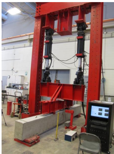
c) Splice test setup with specimen loaded
