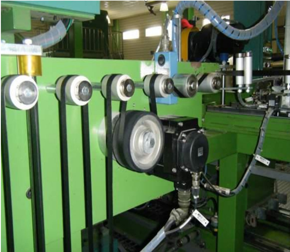
Figure 1. Rubber coated nylon ply tension control mechanism.
