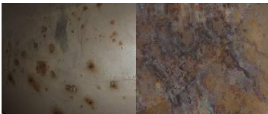
Figure 2. Field images of the outer (left) and inner (right) surface of Type 201 steel tank in Hai Phong.
