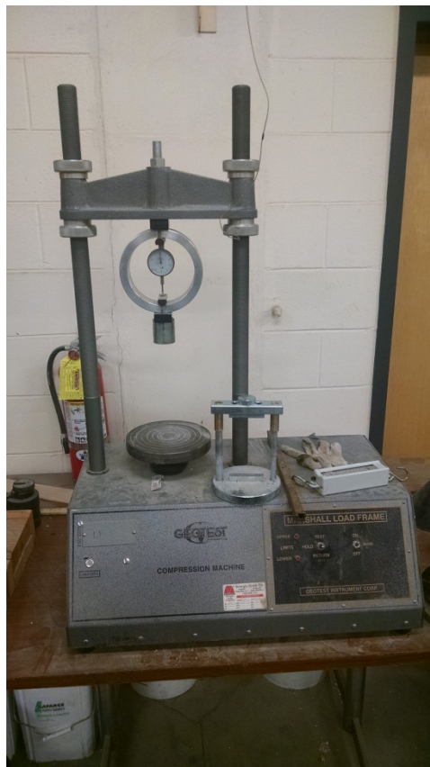
Figure 3.18. Geotest compression machine and modified Lottman breaking head
