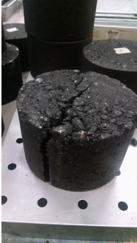
Figure 5.27. Typical failure of ITS samples
