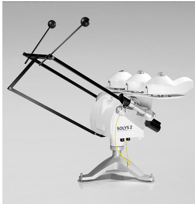
Figure 4: Kipp & Zonen SOLYS 2 Solar Tracker and Irradiance Equipment
