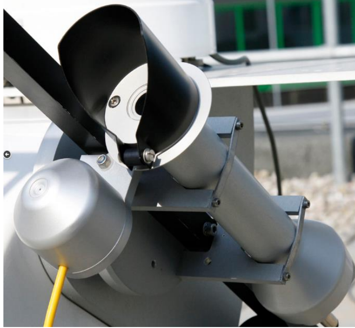
Figure 12: Pyrheliometer and Sun Sensor Mounted to Side Plate of the SOLYS 2
