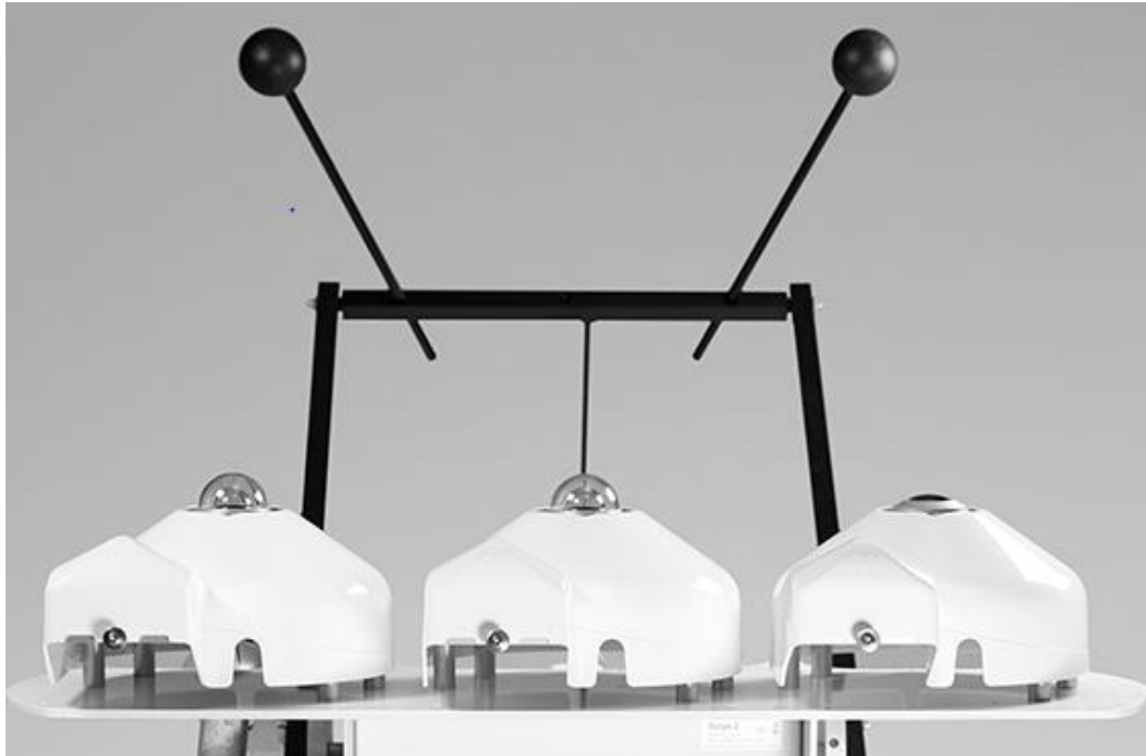
Figure 13: Shaded Pyranometers, Un-shaded Pyranometer, and Shaded Pyrheliometer Mounted Respectively on the Top Mounting Plate of the SOLYS 2
