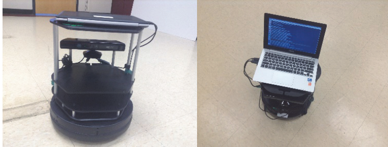
Figure 3.1 The Turtlebot with Kinect and Laptop
