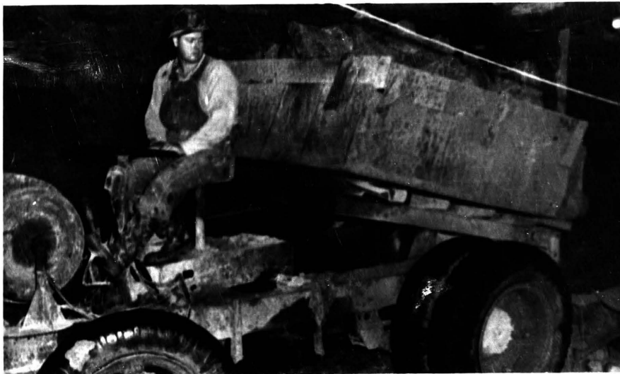
Fig. 3 Electric dump truck discharging an 8-ton ore load. The cable-reel spools 500 feet of 3-conductor No. 6 cable for the 15 h.p. induction motor which is mounted below the reel. A Model 55 White truck chassis has been shortened by three feet. Two truck transmissions are used as speed-reducers, coupled directly to the motor, which has a speed of 900 rpm.
