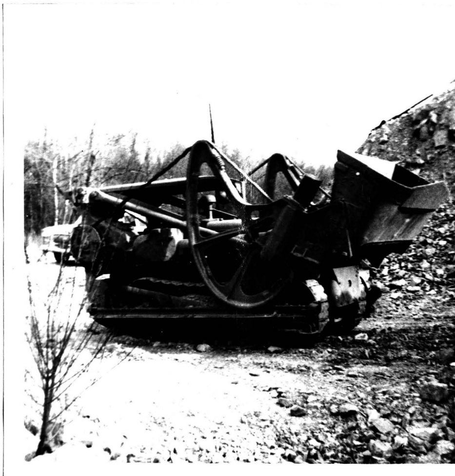
Fig. 5 A Model 102 Eimco diesel over-head loader built on a D-2 Caterpillar tractor chassis, and powered by a 38 h.p. Caterpillar diesel engine. It has a three-quarter cubic yard digging bucket.
