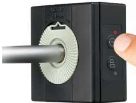
Figure 3.8. Microphone inserted in to calibrator (Kjær, Sound Calibrator Type 4231 n.d.)
