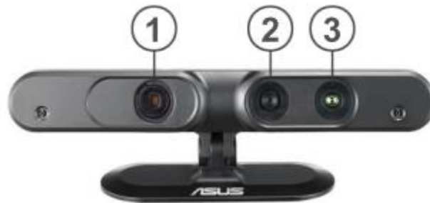
Figure 9: ASUS Xtion PRO LIVE camera: 1 IR projector 2 RGB camera 3 IR camera
