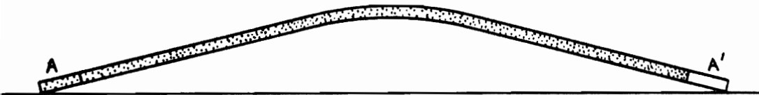
FIG. 11 . GLASS TUBE SHOWING GROUND DOLOMITIC LIMESTONE INTRODUCED AT "A" AND "A'" THE SYSTEM WAS FILLED WITH OIL SOAKED SAND AND ACIDIFIED SEA WATER.
