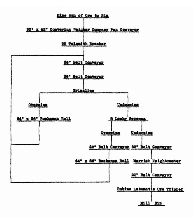
Flow Sheet of Design Consolidated Lead Company's Course Grunning Plant.
