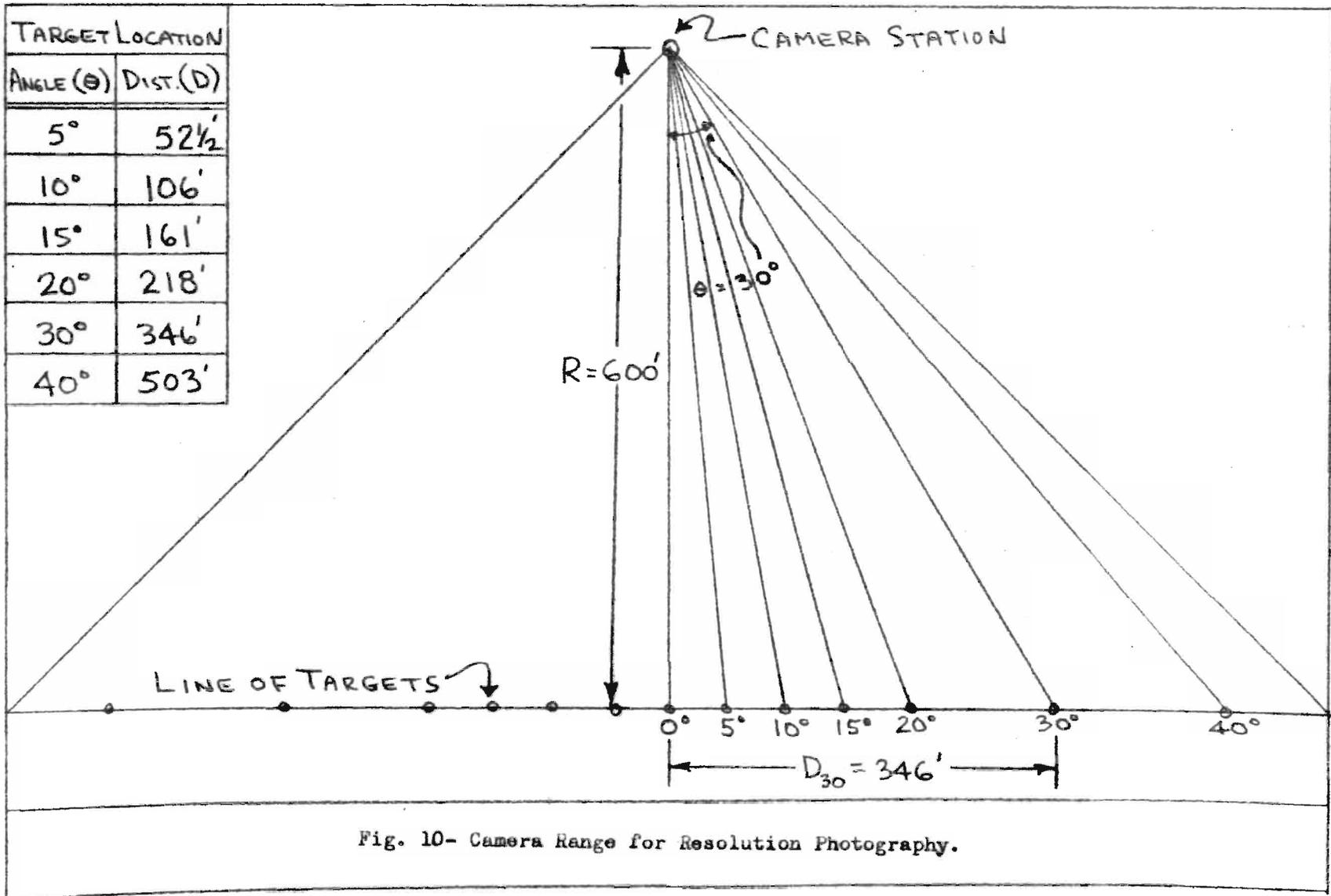
Fig. 10- Camera Range for Resolution Photography.
