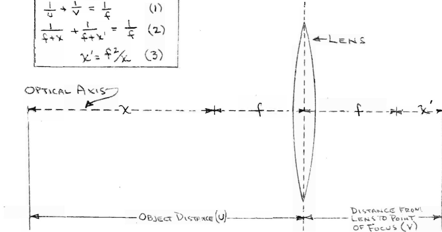
Fig. 15 - Relation of Object Distance to Position of Focus.
