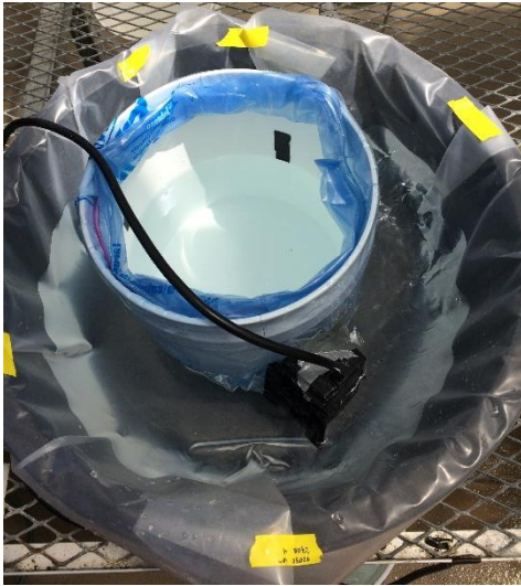
Figure 1: Stream mesocosm with a powerhead pump attached to the side of the bucket generating a recirculating flow of 0.1 \text{ m s}^{-1} . The water inside the bucket serves as a lentic system.
