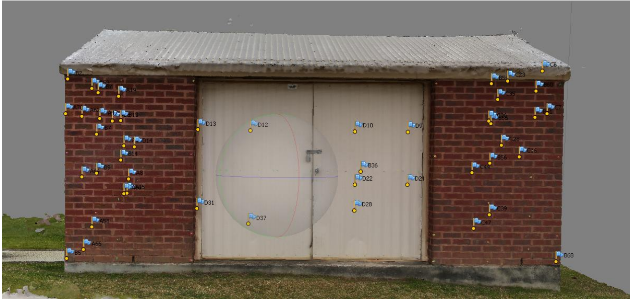
Figure 4.11 Points marked on RAC storage building model
