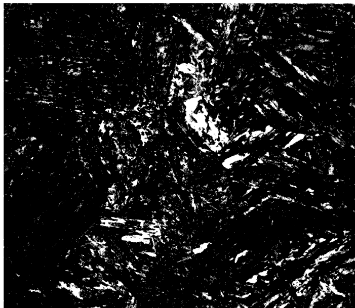
Figure 20. Sample 6SV. As-quenched structure. Austenitized at 1700°F for 1 minute. Nital etch. 500x
