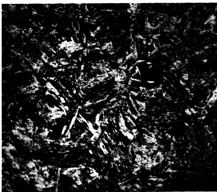
Figure 7. Sample 1KZ. As-quenched structure. Austenitized at 1650°F for 3 minutes. Nital etch. 500x
