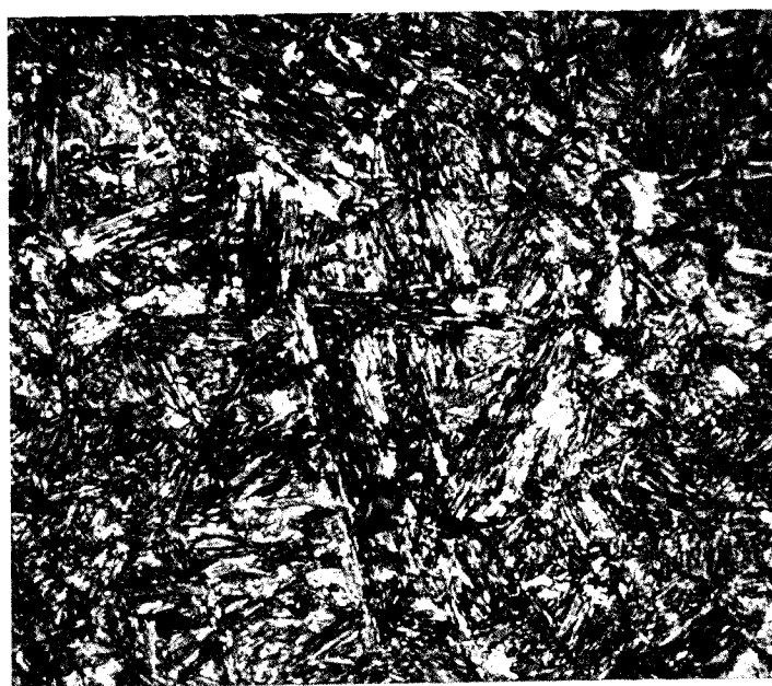
Figure 9. Sample 1SZ. As-quenched structure. Austenitized at 1700°F for 3 minutes. Nital etch. 500x
