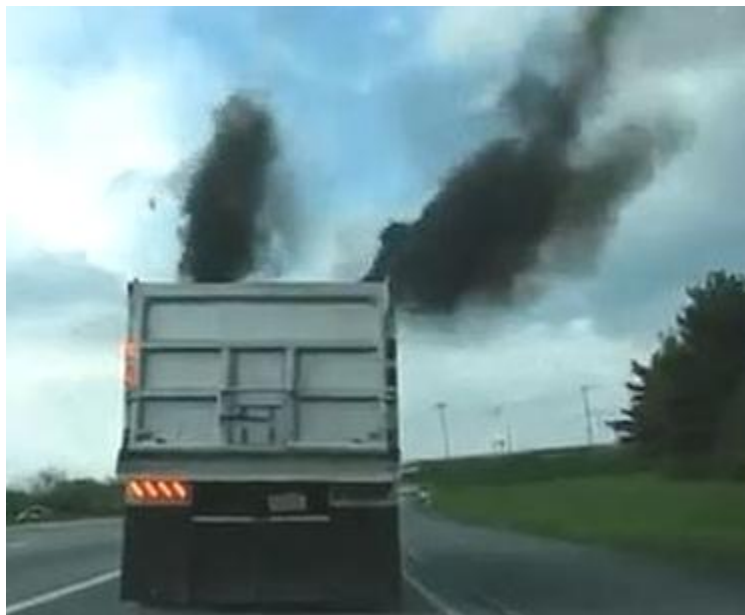
Figure 3: Emission of soot while accelerating under load. [11]
