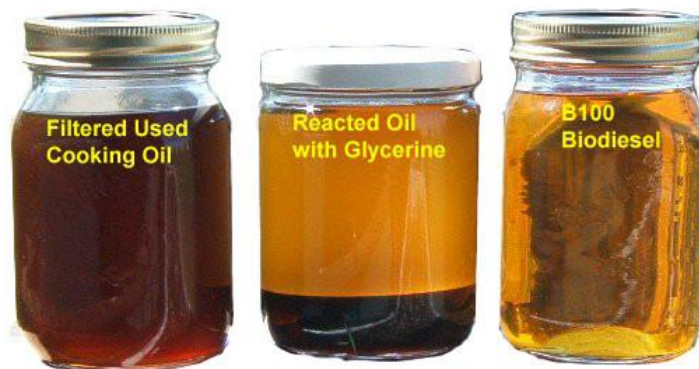
Figure 10: Biodiesel from feedstock to finished B100
