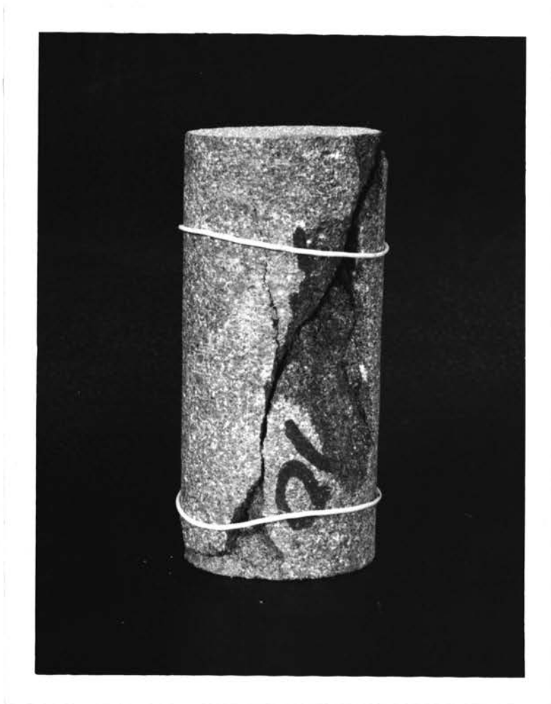
Figure 43 Compressive Failure of a White Pine Sandstone Sample Under a Condition of 4eE-70^\circ .
