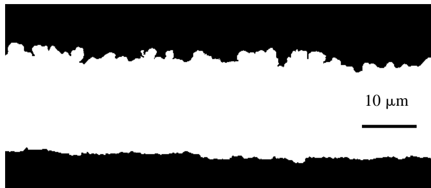
Figure 3.20. Binary image of the cross-section for VLP
