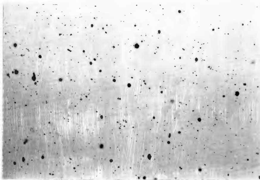
Figure 4la. Armco iron punching. Transverse.
