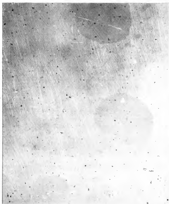
Figure 51. Ingot No. 13, bottom. As cast. Transverse. 150 X; Unetched
