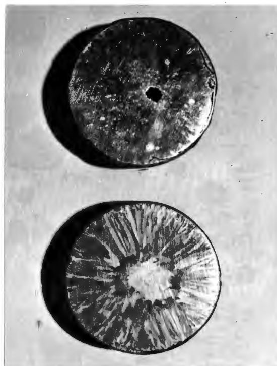
Figure 32. Ingot 11, macro-etched sections. Ingot top, above; bottom, below. 10% Nital, 2 minutes
