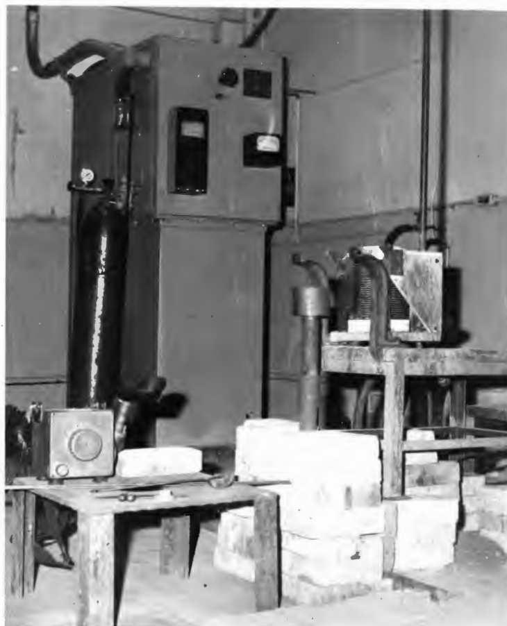
Figure 7. Furnace assembly and converter unit.
