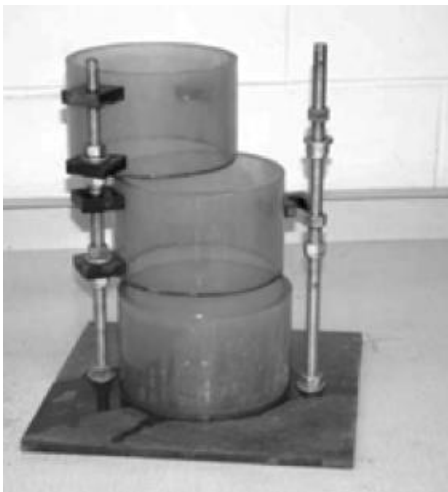
Figure 3.17 Three compartment hinged cylindrical mold [10].
