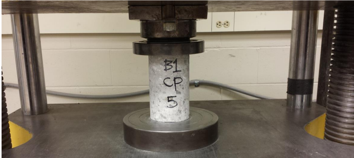
Figure 5.19 Compressive strength test setup of cores.
