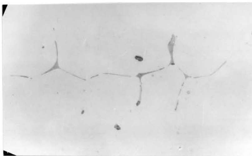
Figure 28. Sulfide Inclusions In H4 Steel Ingot. Unetched, 500X
