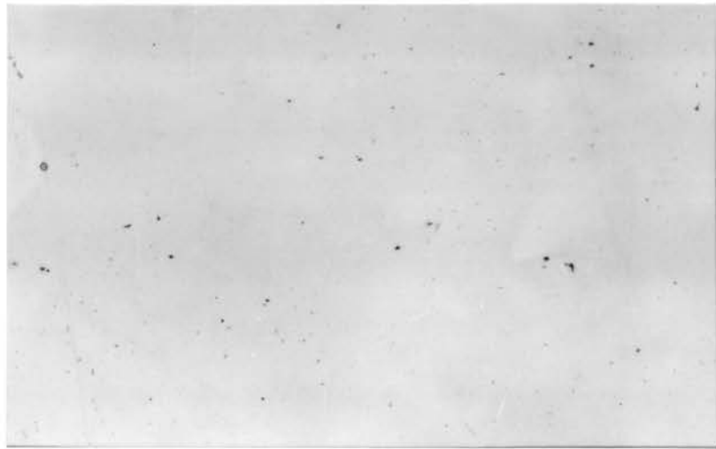
Figure 36. Inclusions In 1042 Steel Wrought Bar. Unetched, 250X
