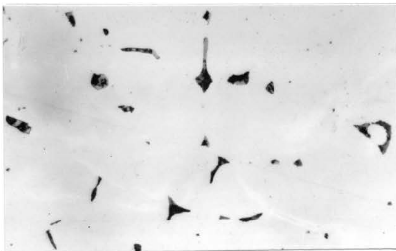
Figure 29. Sulfide Inclusions In H4 Steel Ingot Sample After Test. Unetched, 500X
