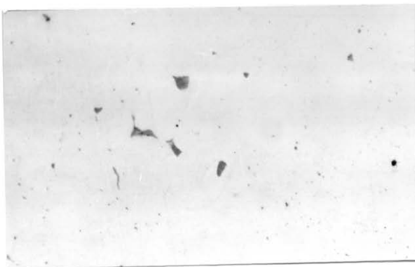
Figure 31. Sulfide Inclusions In H7 Steel Ingot Sample After Test. Unetched, 500X
