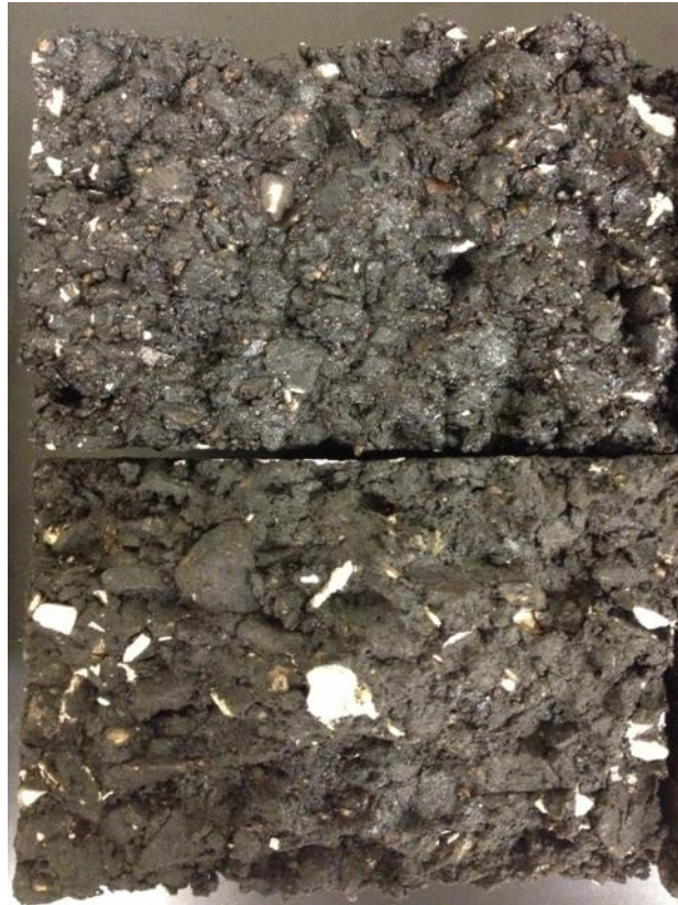
Figure 4.10 – JCD-12 Unconditioned Top/Conditioned Bottom
