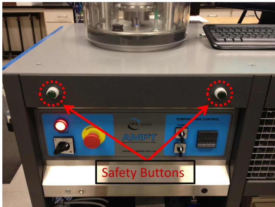
Figure 8 – External Lowering Safety Buttons
