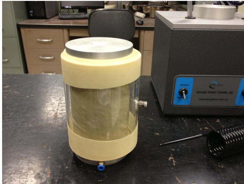
Figure 3.23 - Latex Wrapped Specimen for Flow Number Test
