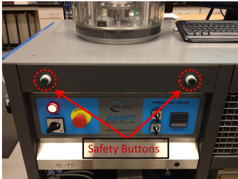
Figure 4 – External Lowering Safety Buttons
