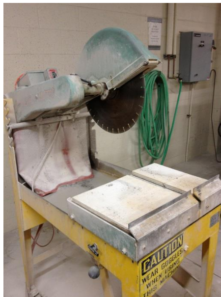
Figure 1 - Wet Saw with Diamond Cutting Blade
