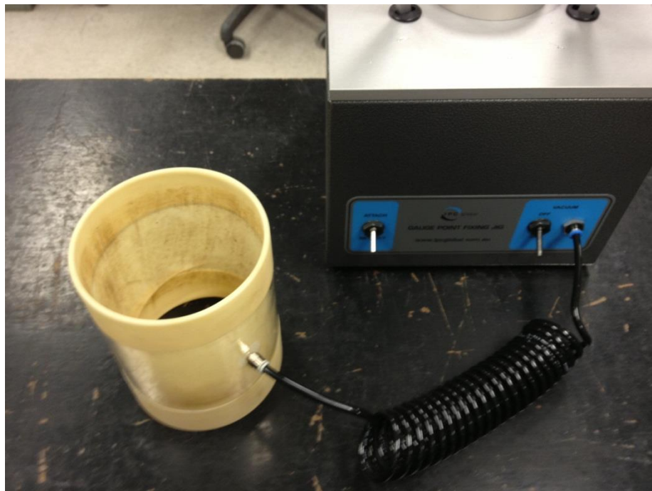
Figure 1 – Membrane Over Collar with Vacuum Applied
