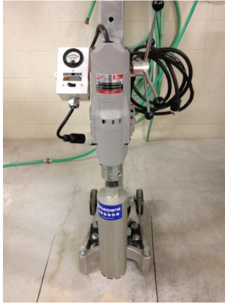
Figure 1 - Core Drill with Diamond Bit
