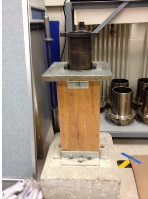
Figure 3 – Mold Secured in Compaction Pedestal
