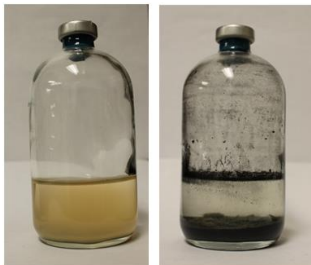
Figure 5.1 Left: Serum bottle without black precipitate (switch grass) Right: Serum bottle with black precipitate (sweet potato).
