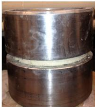
Figure 5.6.4 Shear ring without spacer
