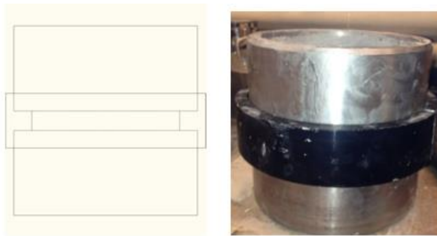
Figure 5.7.2 Direct shear test sample
