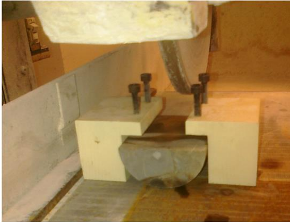
Figure 4.5.3 Grinding Desired Fracture Width
