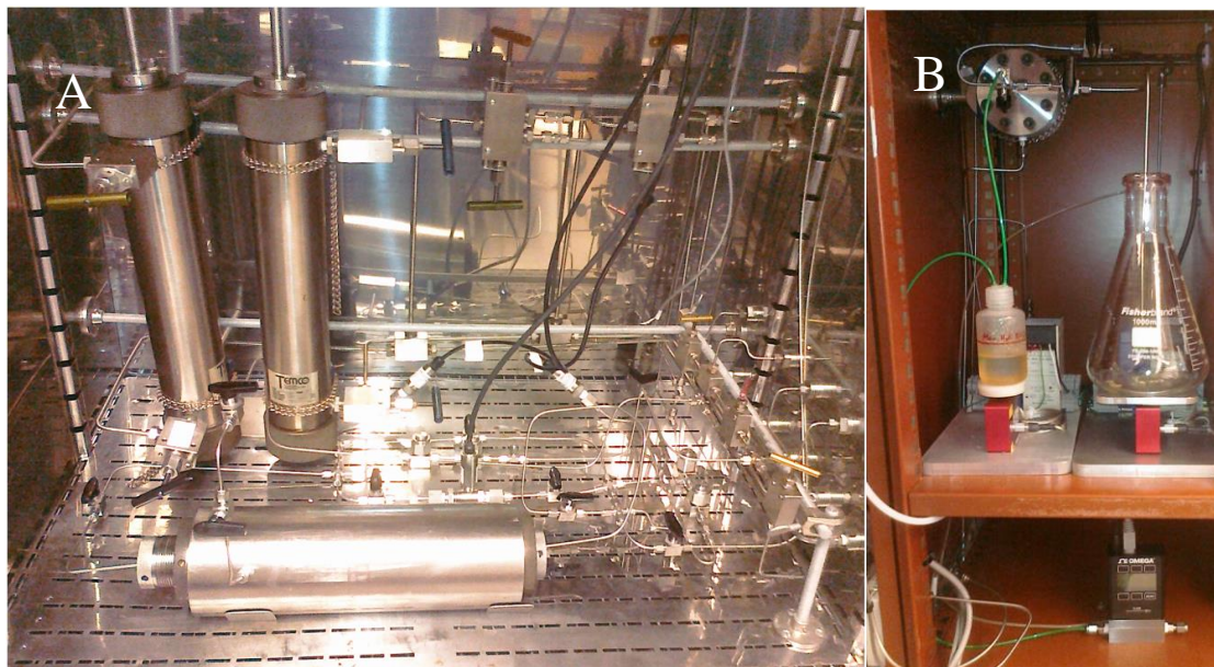
Figure 5.0.2 Core Flooding System Setup
