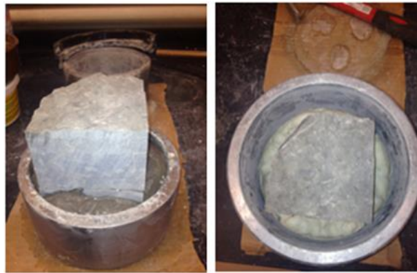
Figure 5.6.3 Rock sample in shear ring
