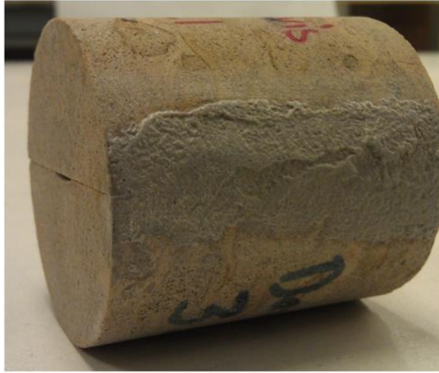
Figure 4.5.4 Fractured core held together with epoxy
