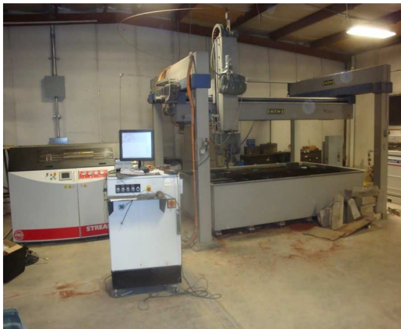
Figure 3.1. The 5-axis PaR system coupled with the 125Hp intensifier
