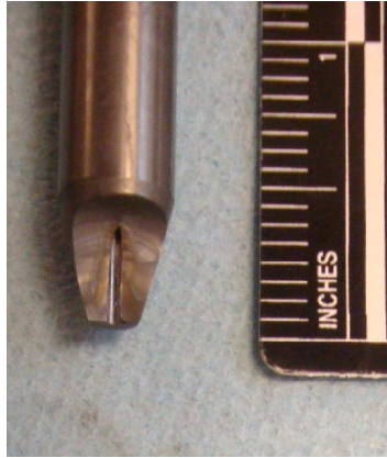
Figure 4.15. Damaged Focusing Tube
