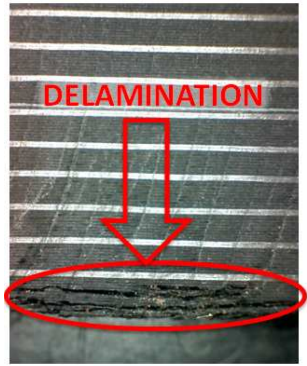
Figure 4.2. Delamination of 1" composite cut at 50,000psi (25x)
