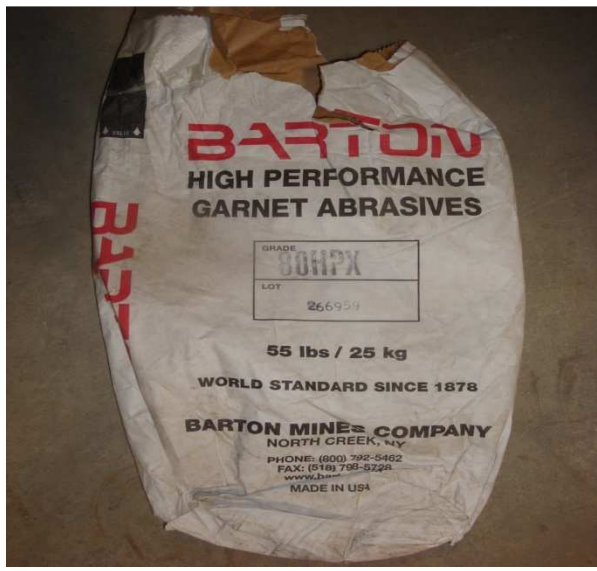
Figure 3.8. 80HPx abrasive with batch number
