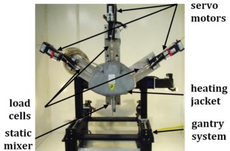
Figure 2.1. The triple-extruder Freeze-form Extrusion Fabrication (FEF) machine.
