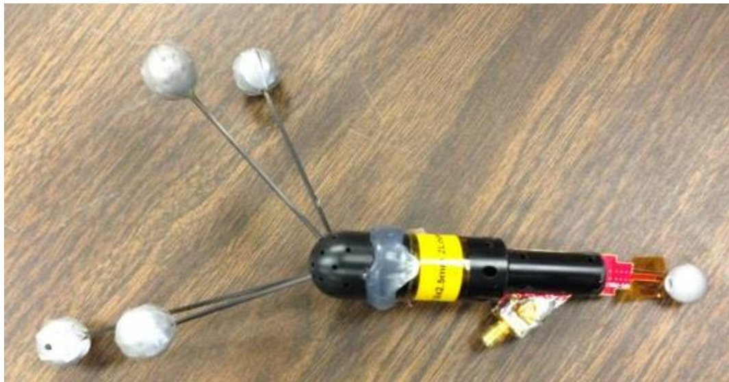
Figure 2.50. Rigid body and probe with an extra marker at the tip of probe
