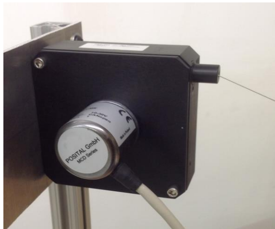
Figure 2.3. Draw wire sensor
