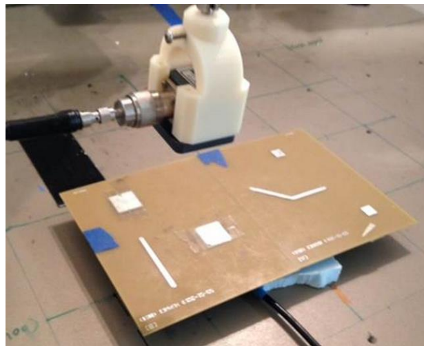
Figure 4.10. Custom board with a waveguide above
