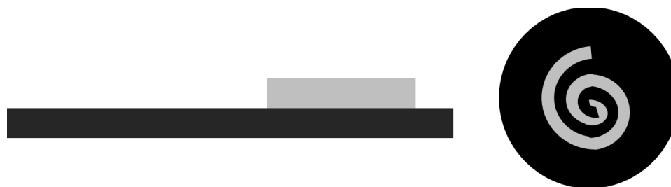
Figure 1. Schematic of the initial sheet layup which is then rolled up to the final spiral formation where the light gray is SiC and the black is \text{TiB}_2 .
