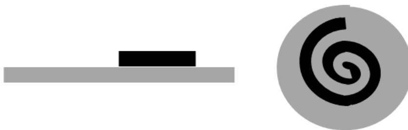
Figure 1. Schematic of the initial sheet layout which is then rolled up to the final spiral formation where the light gray is SiC and the black is TiB 2
