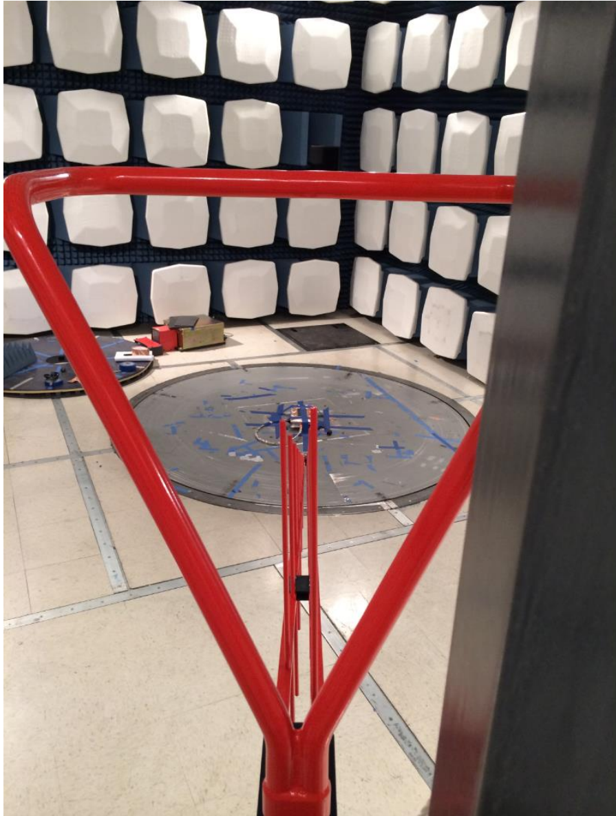
Figure 5.6. Far field measurement setup
