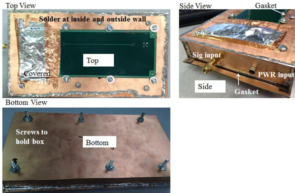
Figure 5.4. Different views of the shield box
