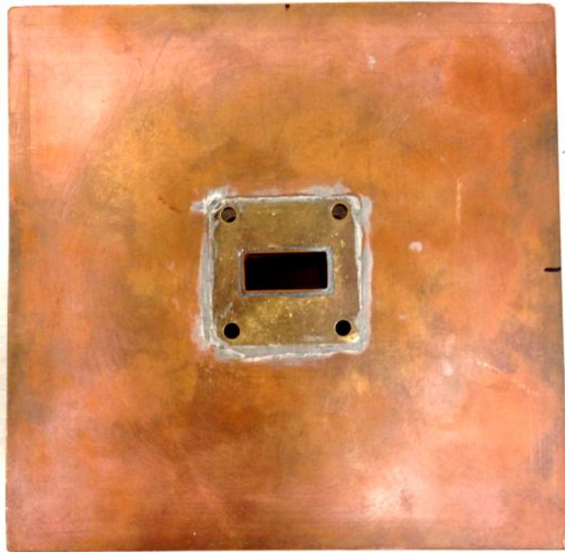
Figure 4.9. Custom-made large flange (152 mm x 152 mm).
