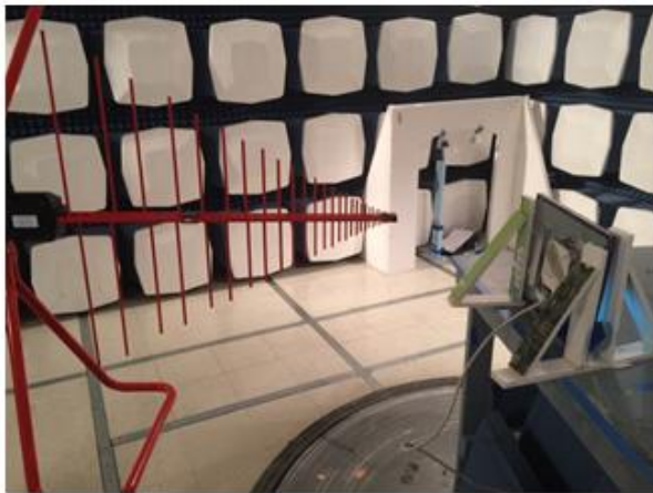
Figure 1.23. Far Field measurement of the computer screen in the 3 m chamber.
