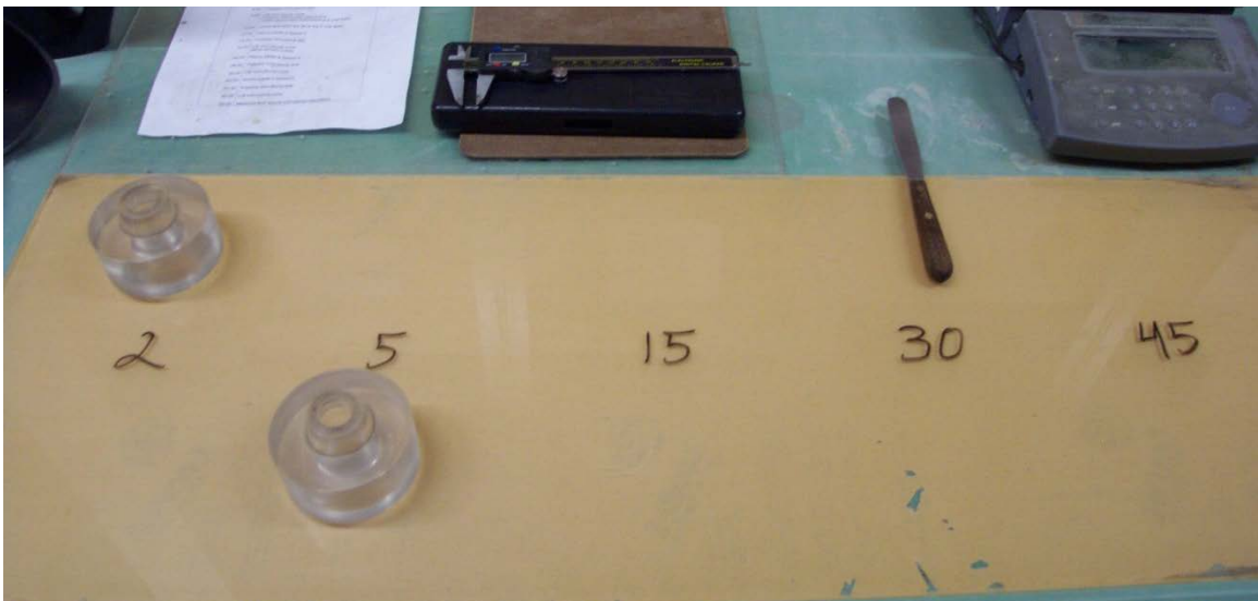
Figure 3.6. Miniature Slump Cones and Equipment
