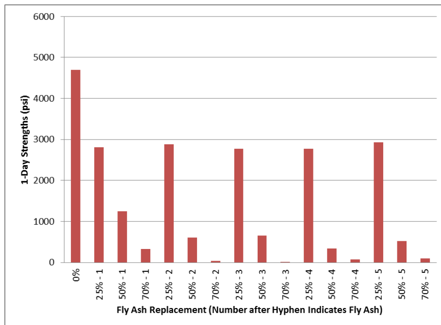
Figure 4.1. One-day Compressive Strengths for Cement 1 Combinations
