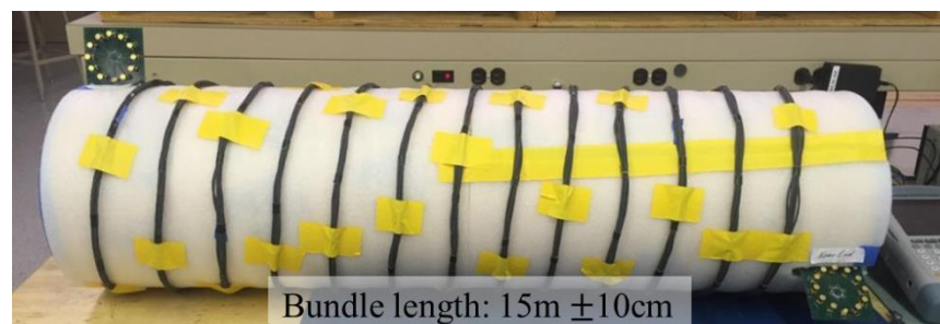
Figure 3.5. Measurement setup for Leoni Dacar 545 cable bundle
