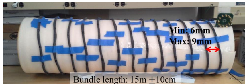
Figure 3.4. Measurement setup for Leoni Dacar 546 cable bundle
