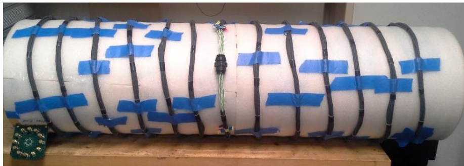
Figure 3.15. Measurement setup for Leoni Dacar 546 cable bundle with an inline CPC with maximum 25 cm untwisted segment
