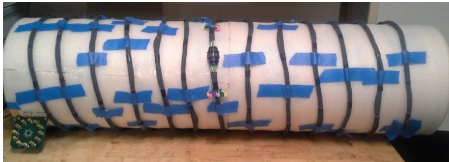
Figure 3.14. Measurement setup for Leoni Dacar 546 cable bundle with an inline CPC with minimum 7 cm untwisted segment
