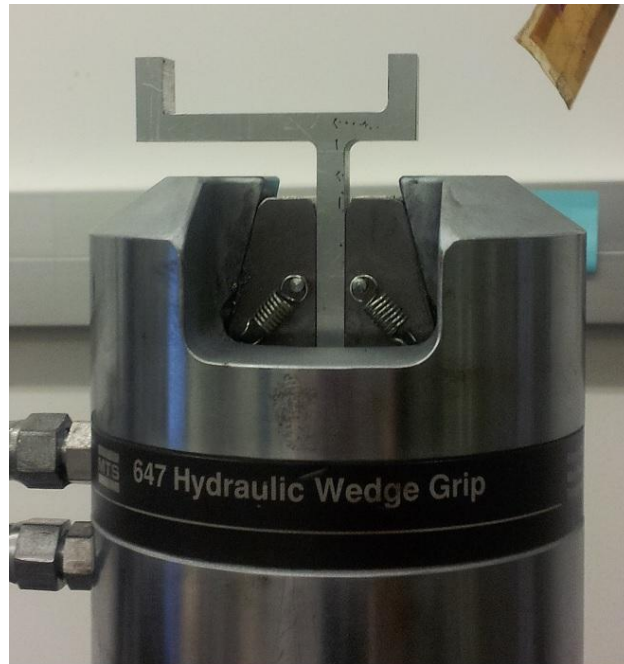
Figure 5.5 – Eccentric Fixture used in Conjunction with Blade Design 1.0 to Prevent Blade Twisting
