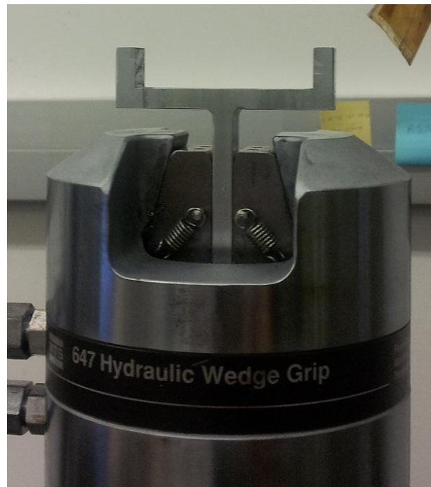
Figure 5.6 – Centric Fixture used in Conjunction with Blade Design 1.1 and 1.2 to Prevent Blade Twisting
