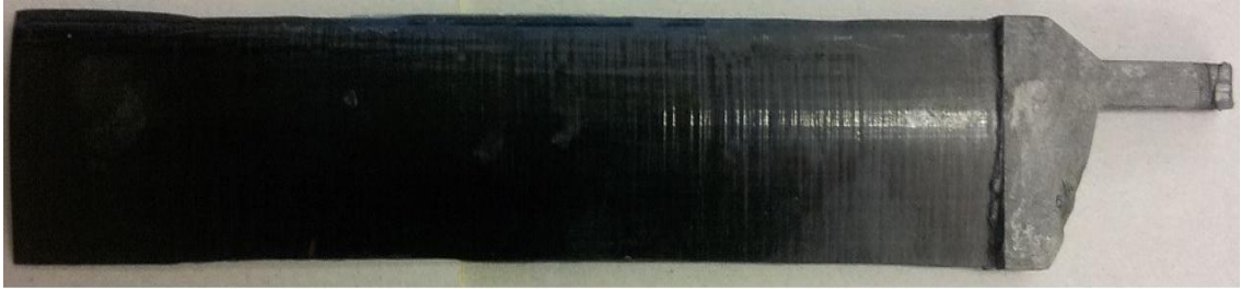
Figure 3.5 – Composite Blade Design 1.1 with Metal Epoxy Tabs Cured to Root and the Area Leading to the Constant Area Cross Section
