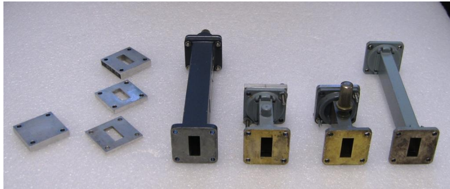
Figure 3.4. The Calibration loads and DUTs used to test the X-band VNA - in order: short, shims (3 mm, 5 mm and 9 mm), matched load, two attenuated shorts (variable and 3 dB) and an open-ended waveguide radiating into air.
