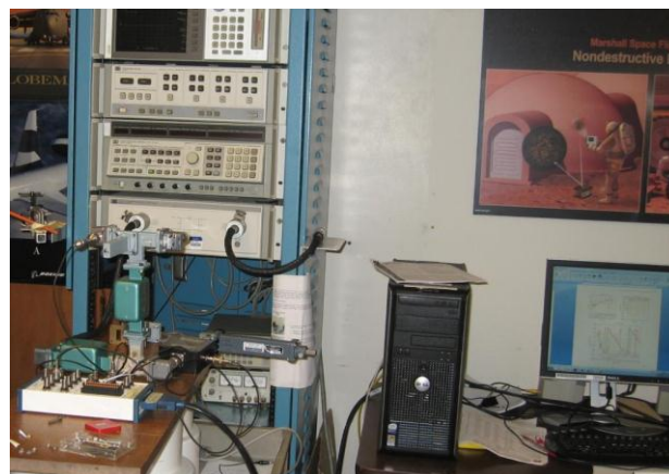
Figure 5.25. Setup to perform measurements using a Magic-T.
