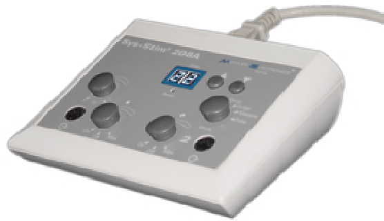
14. SyStim 208. Neuromuscular Stimulator for electrical stimulation therapy. This is a portable unit that would be taken from storage when use what needed.
