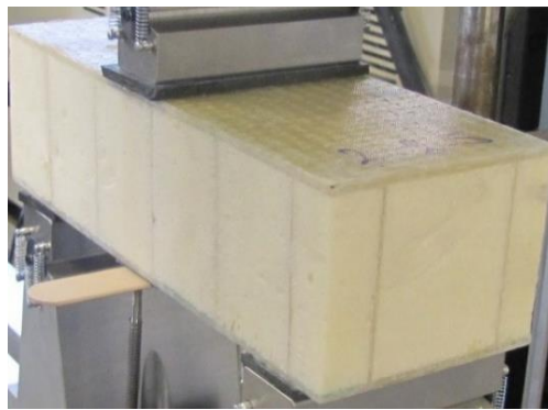
Figure 5.2: Three Point Flexural Test Specimen for Type 2
