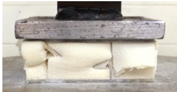
Figure 4.12: Damage at End of Test for Flatwise Compression Testing on Type 2
