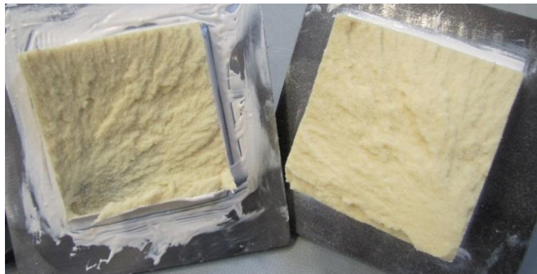
Figure 4.19: Fracture at the End of Test for Flatwise Tension Testing on Type 1
