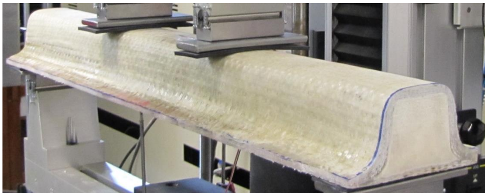
Figure 5.21: Four Point Flexural Test Specimen for Type 3
