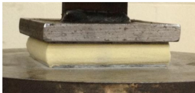
Figure 4.9: Damage at End of Test for Flatwise Compression Testing on Type 1
