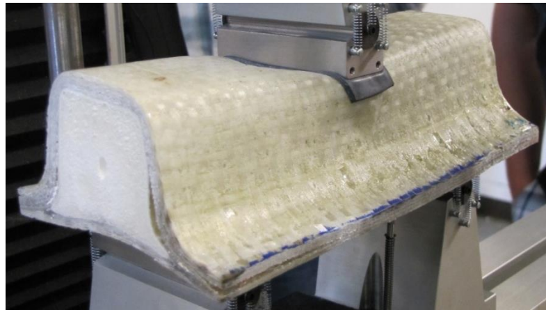
Figure 5.16: Three Point Flexural Testing Initial Failure by Delamination Between the Shear Layers for Type 3
