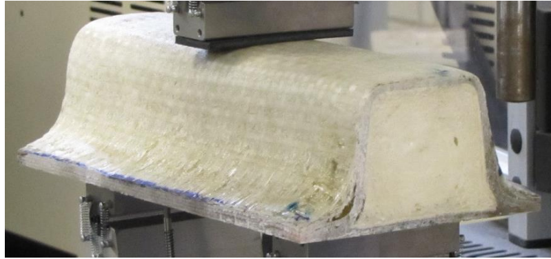
Figure 5.3: Three Point Flexural Test Specimen for Type 3
