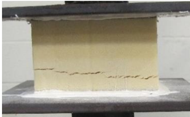
Figure 4.18: Damage at Failure for Flatwise Tension Testing on Type 1
