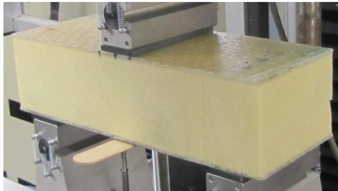
Figure 5.1: Three Point Flexural Test Specimen for Type 1
