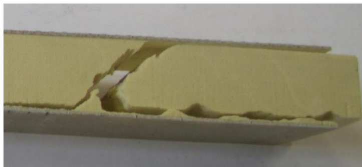
Figure 5.28: Four Point Flexural Testing Ultimate Failure Due to Shear Failure in the Core Material for Type 1
