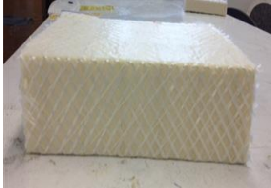
Figure 3.2: Raw Material Block of the Type 2 Core
