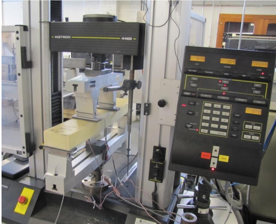
Figure 5.22: Test Setup Used for the Four Point Flexural Test
