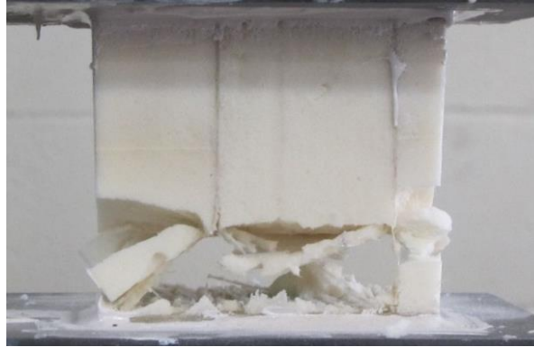
Figure 4.22: Damage During Bond Failure for Flatwise Tension Testing on Type 2
