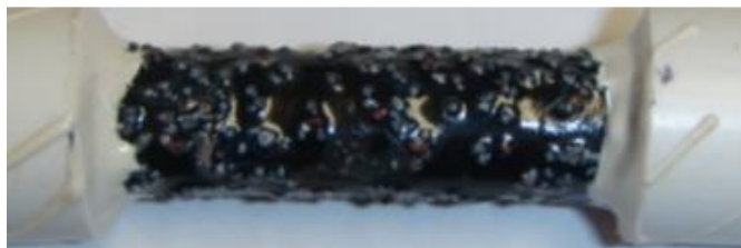
Fig.2. Sand particle-modified enamel coated steel bar.
