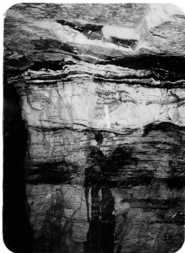
Fig. 5. - Two types of arkosic sandstone and their relation with uranium-vanadium content, 500 stope, Becenti ore body.
