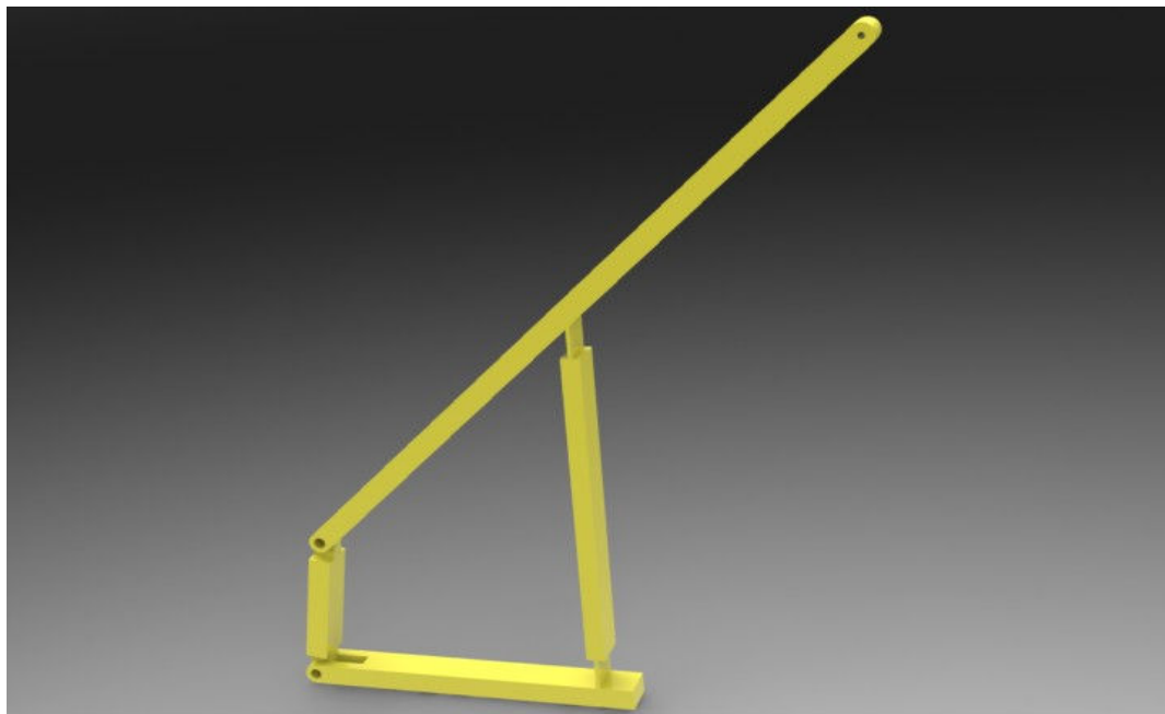
Figure 4.12. Solid Model of Compliant Straight-Line Generating Mechanism with Two Small-Length Flexural Pivots
