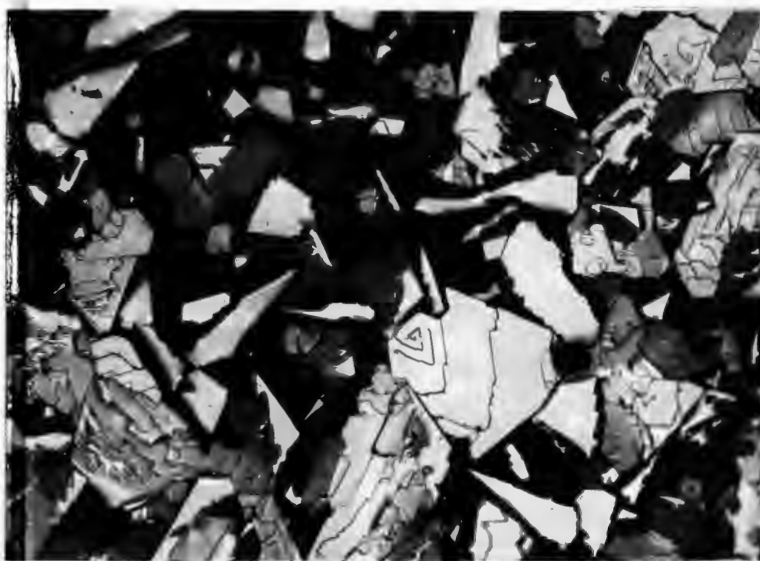
Figure 22. Nickel oxide on INCO HPM Ni oxidized at 1300° C. Sample F-24, unetched, 250X.
