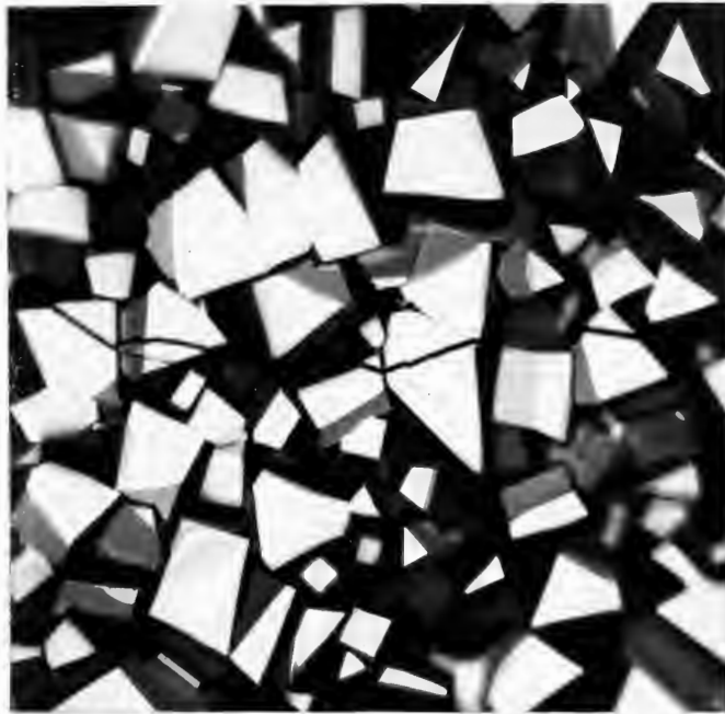
Figure 20. Cracked nickel oxide on INCO HPM Ni oxidized at 1300° C. Sample F-26, unetched, 500X.
