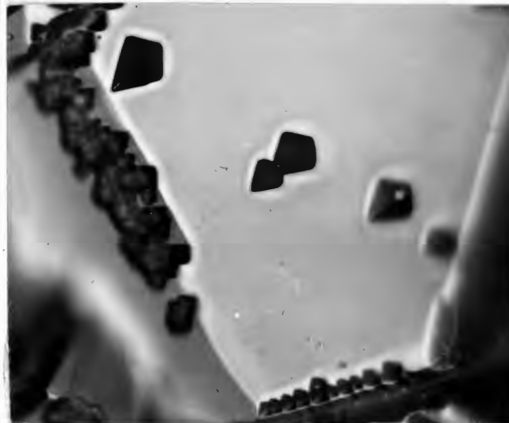
Figure 15. Etch pits in nickel oxide on low purity nickel oxidized at 1200° C. for 60 days. Unetched, 2000X.
