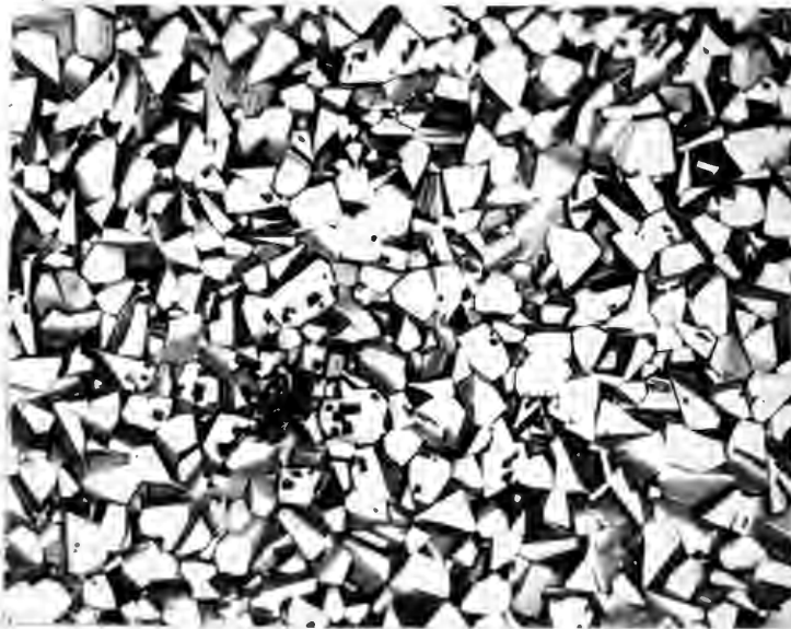
Figure 13. Etch pits in nickel oxide on Foundry Ni oxidized at 1200° C. Sample F-16, unetched, 500X.
