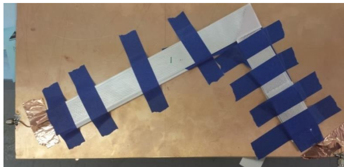
Figure 4.34. Flex cable over copper sheet
