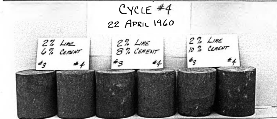
WET DRY TEST CYCLES 1 THRU 4 2% LIME 6-10% CEMENT
