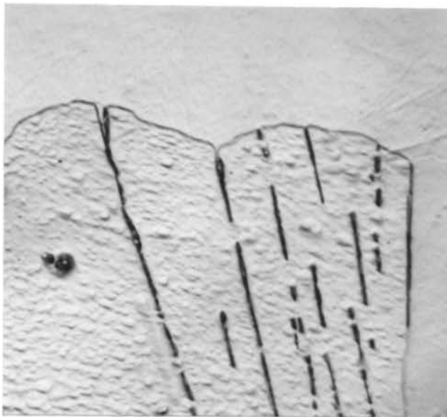
Figure 2. Cell boundary of Pb-3.0 wt% Sn alloy after aging for 360 hours at 23°C. Note that the \alpha' lamellae (light gray) precede the \beta tin lamellae (dark). X500
