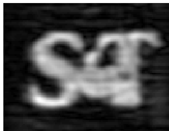
Figure 3.19. Logo scanned with 1 inch-thick rubber sheet covering.
