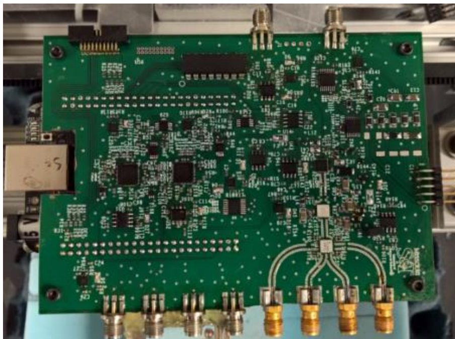
Figure 2.29. Fabricated controller board.
