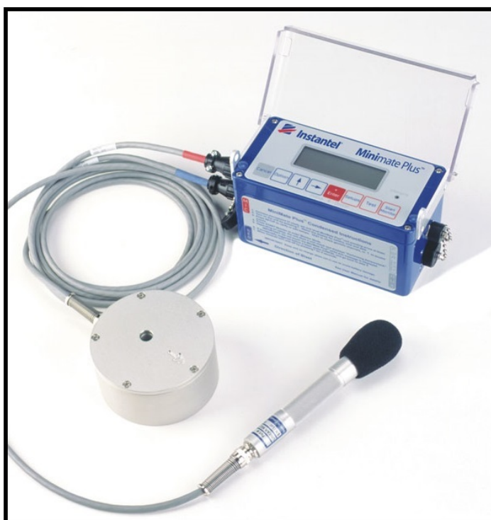
Figure 3.2. Modern Seismometer with Geophone and Microphone
